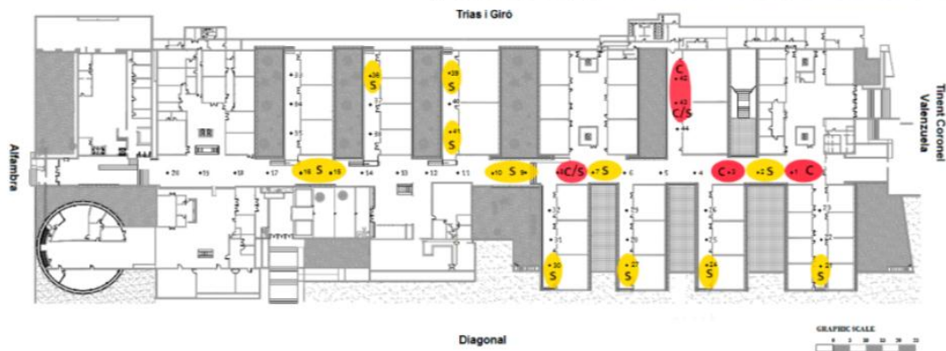
Plan 1: Economics and Business Faculty luxometric plan. Red: luxometric values below norm reference values.
